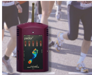
Dynamic pressure measuring between foot and shoe
