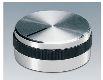
A1432469 TUNING KNOB, with lateral screw fixing ABS (UL 94 HB) brilliant 31.9x14mm 6mm
