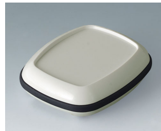
B1604217 BODY-CASE M, with recess ASA (UL 94 HB) traffic white RAL 9016 50x41x16mm IP 65
