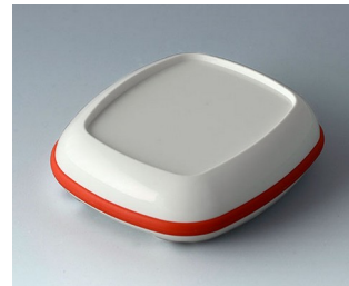
B1606207 BODY-CASE L, with recess ASA (UL 94 HB) traffic white RAL 9016 55x46x16mm IP 65
