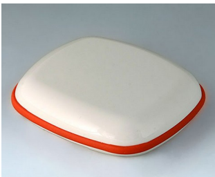
B1608107 BODY-CASE XL, without recess ASA (UL 94 HB) traffic white RAL 9016 62x56x18mm IP 65
