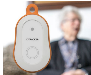
LoRa GPS tracker with alarm button
