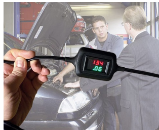
Voltage and current display during trickle charging
