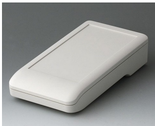
A9006107 DATEC-COMPACT M ASA+PC (UL 94 V-0) off-white RAL 9002 172x92x39mm IP 65
