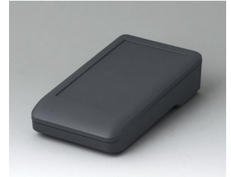
A9005118 DATEC-COMPACT S ASA+PC (UL 94 V-0) lava 136x74x32mm IP 41
