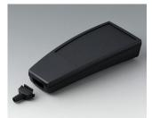
A9068329 SMART-CASE XL, Vers. III ABS (UL 94 HB) black RAL 9005 168x74.4x35.4mm IP 65 opt., IP 40
