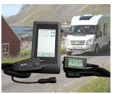
System for leak detection in leisure vehicles
