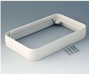
A9153017 Intermediate ring XL ABS (UL 94 HB) off-white RAL 9002 96x154x26mm
