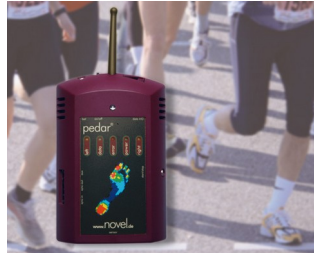
Dynamic pressure measuring between foot and shoe
