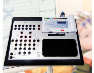
Stationary system for long-term EEG recordings
