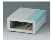
B2213015 MEDITEC E 160, without handle bar ABS (UL 94 HB) off-white RAL 9002 160x200x74mm IP 40
