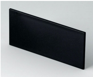
B6121221 Front panel PPO (UL 94 V-0) black RAL 9005 67.8x31.7x2mm
