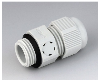
C2316917 Cable gland M16x1.5, pressure compensation PA 6 (UL 94 V-0) light grey RAL 7035 IP 68
