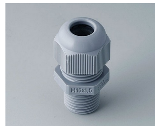
C2316618 Cable gland M16x1.5 PA (UL 94 HB) silver grey RAL 7001
