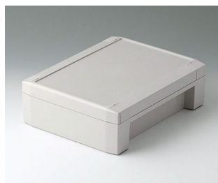
C8017222 SOLID-BOX 175 PC+ABS (UL 94 V-0) light grey RAL 7035 225x175x70mm IP 66, IP 67, IK 08
