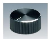
A1418260 TUNING KNOB, with lateral screw fixing ABS (UL 94 HB) black/alu 18.6x12mm 6mm
