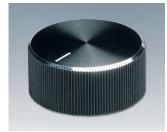
A1432260 TUNING KNOB, with lateral screw fixing ABS (UL 94 HB) black/alu 33x14.3mm 6mm
