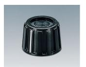
A1319260 TUNING KNOB, with lateral screw fixing black RAL 9005 18.9x13.5mm 6mm
