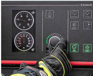
Control element for pump control station
