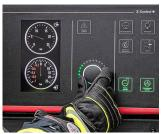
Control element for pump control station
