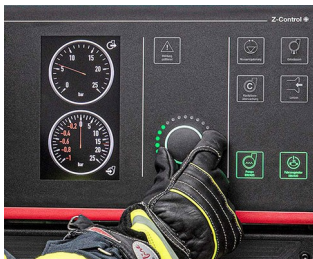
Control element for pump control station
