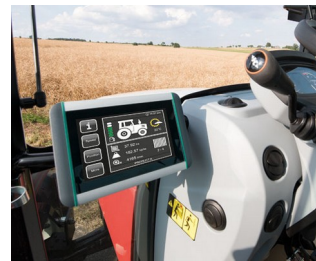
ISOBUS terminal for tractors and self-propelled machines
