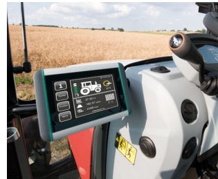
ISOBUS terminal for tractors and self-propelled machines
