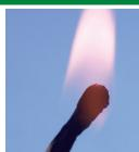
Test: The test samples are extinguished within 50 seconds average time (mean of 10 successive tests). None of the test samples burns longer than 10 seconds. None of the test samples emits burning particles.
